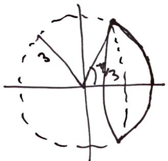
$$\begin{aligned} S &= 2\pi \int_a^b y \, ds \\ &= 2\pi \int_a^b y \sqrt{x'^2 + y'^2} \, dt \\ &= 2\pi \int_0^{\frac{\pi}{3}} 3\sin x \sqrt{(-3\sin x)^2 + (3\cos x)^2} \, dt \\ &= 18\pi \int_0^{\frac{\pi}{3}} \sin x \, dt \\ &= 18\pi [-\cos x]_0^{\frac{\pi}{3}} \\ &= -18\pi [\cos \frac{\pi}{3} - \cos 0] \\ &= -18\pi [ \frac{1}{2} - 1 ] \\ S &= 9\pi \end{aligned}$$
